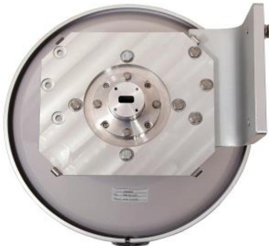
Figure 17: Mounting AL set on parabolic antenna flange
